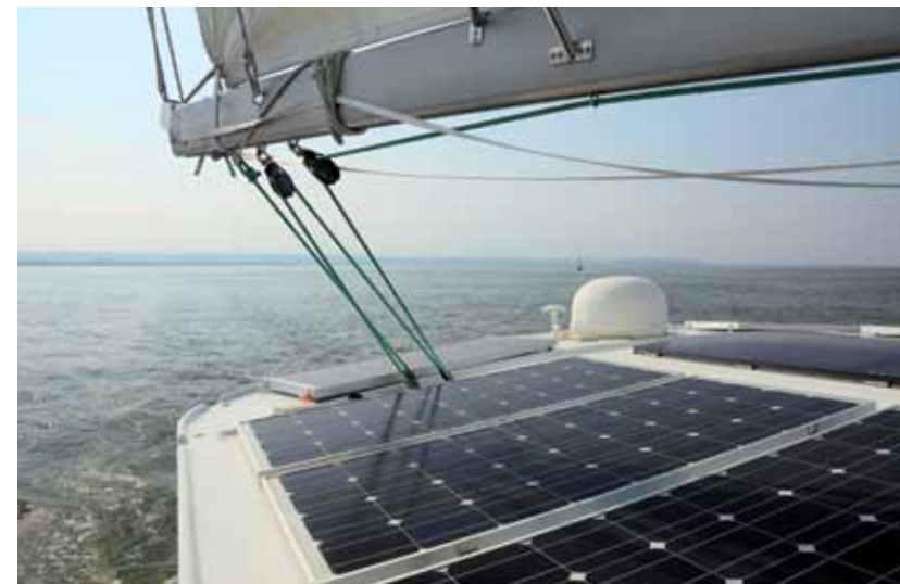
FUEL OF THE FUTURE? Solar-charging batteries aboard a sailboat with photovoltaic panels.
